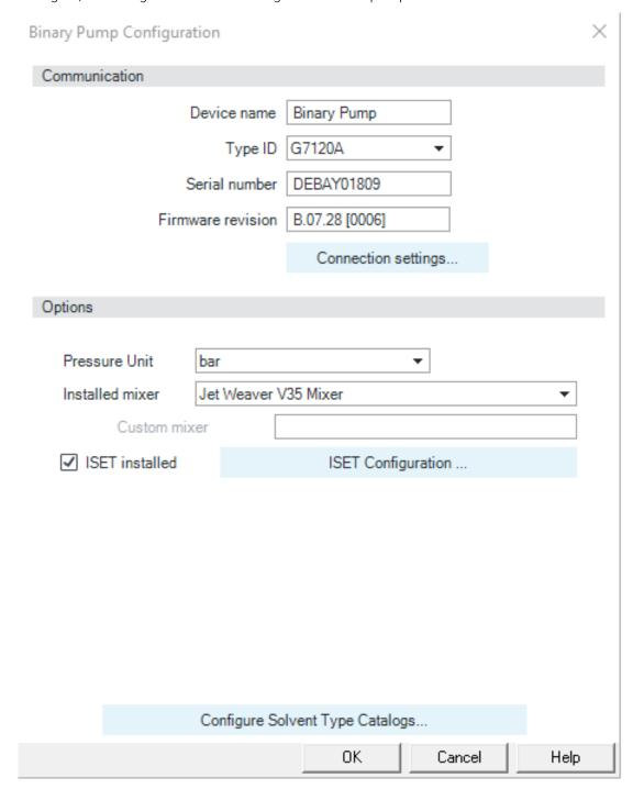
3 In the additional configuration of the pump module, choose Configure Solvent Type Catalogs...
